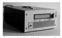
Model AG 1016 Amplifier/ Generator is a robust source of RF power for ultrasonic, laser modulation, RFI/EMI, plasma generation, general laboratory and industrial applications.
